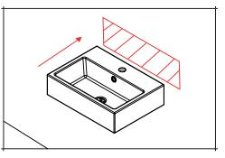
Mount the basin to the wall at your desired height. Our suggested height would be between 800-850mm from the finished floor to the top of the basin.
