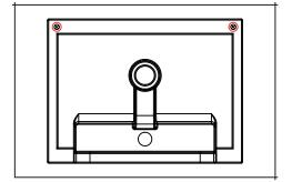
Remove the two bolts from the underside of the basin. Place the screws to one side\*.
