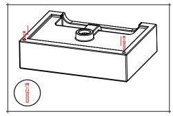
Insert the two brass bolts with a tapered end shown in the diagram, Use a flathead screwdriver to tighten.
