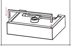
3. Locate the rail onto the brass bolts. Loosen the grub screws slightly with the hex key provided to ensure they do not obstruct the location of the bolts. Ensure the grub screw holes are facing inward towards the back of the basin.
